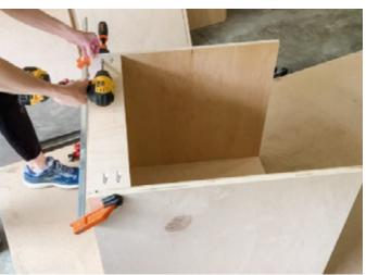
Pocket-hole joinery, or pocket-screw joinery, involves drilling a hole at an angle - usually 15 degrees - into one workpiece, and then joining it to a second workpiece with a special screw. Often used to join boxes together.
