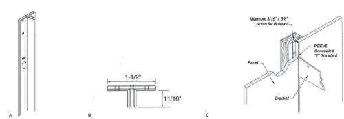
All recessed/ concealed « T » standards should be mounted right side up as shown by the "top" stamp (A). Before mounting, line up each standard using the bottom of each bottom slot as the guide. Once aligned, makes sure to fasten to a secure wall stud (or equivalent blocking) using appropriate screws (C). Make sure to utilize each screw hole. Please note that a minimum 3/16" by 5/8" notch is required in the stud or blocking to allow installation of brackets.
