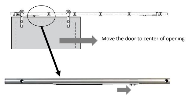
Charge the soft close mechanism by manually pushing the tabs towards the center of the opening until it locks itself to a stop (you will feel resistance)
