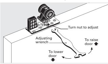
Note: The top of the hanger pin screws into
