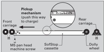
b) Most of the time you will have room to slide the mechanism in from the end of the track fully assembled. c) If there is not enough room, remove the front carriage (attached to the SofStop cassette).
