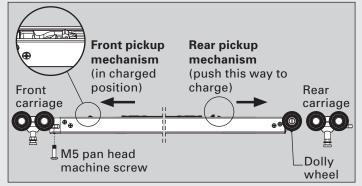
Most of the time you will have the room to slide the mechanism in from the end of the track fully assembled.
