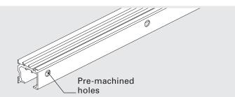
Note: for 2" thick doors, a 6.35mm (1/4") spacer is required. For 2-1/4'' thick doors, a 12.7mm (1/2'') spacer is required. For fixing to concrete walls, the use of masonry anchors is recommended. You may need to open the existing holes to suit the type of masonry anchor you have selected. Clean out all swarf and debris from the track before hanging the door.
