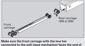
connected to the soft close mechanism faces the end of the track that you want to soft close.
