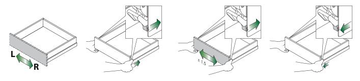
Tilt Adjustment - H90 with Rectangular Railing
