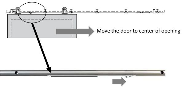
Charge the soft close mechanism by manually pushing the tabs towards the center of the opening until it locks itself to a stop (you will feel resistance)
