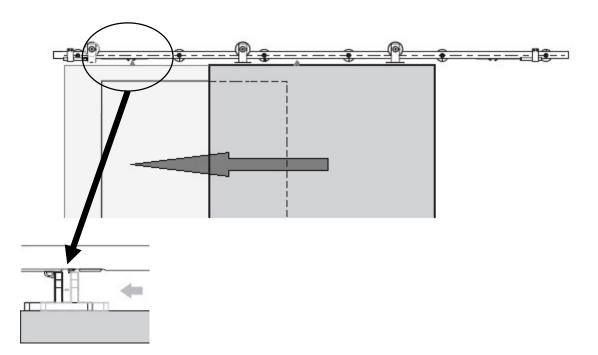
Slide door gently to the left so that it engages with the soft close and fully cycles.
