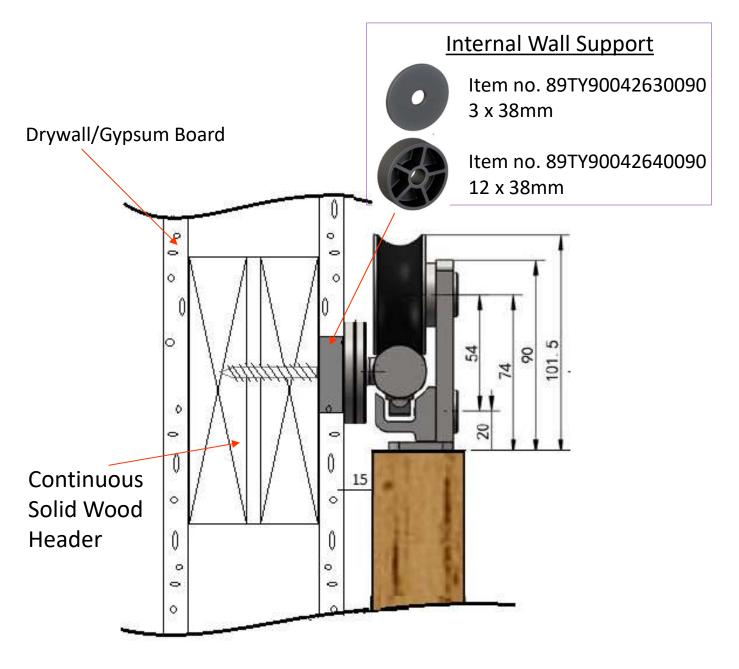
Drill 38mm (1-1/2") hole in drywall/gypsum board and Insert disc(s) to appropriate thickness
