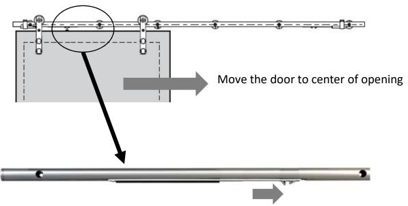
Charge the soft close mechanism by manually pushing the tabs towards the center of the opening until it locks itself to a stop (you will feel resistance)
