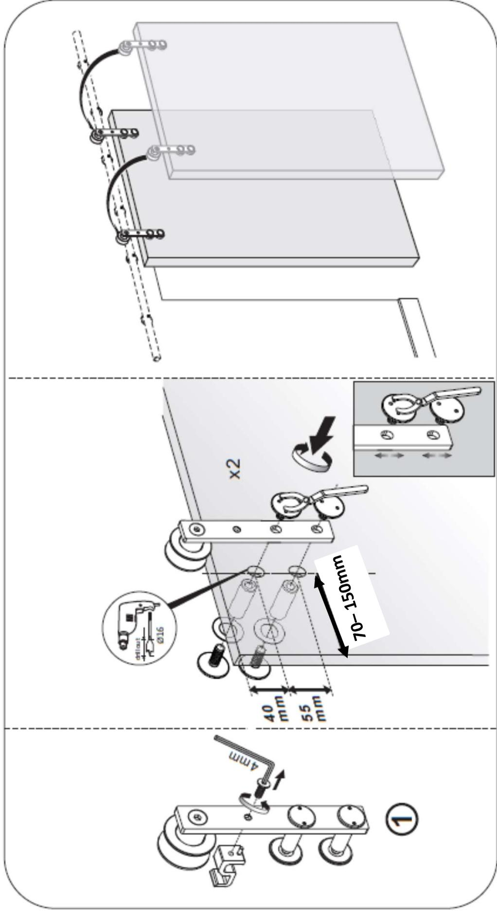
Before mounting the upper trolleys on to the track remove all dust and debris from the track and trolleys. Use a dry cloth, see page 15 for more information.
