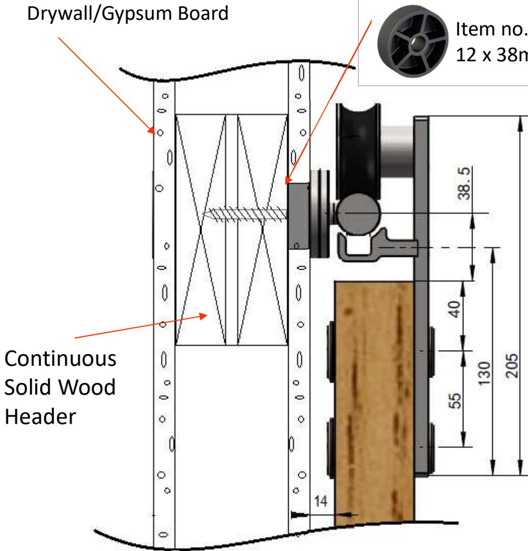
Drill 38mm (1-1/2") hole in drywall/gypsum board and Insert disc(s) to appropriate sheetrock thickness
