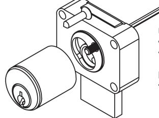
Use a 5/64" Allen wrench from the back to remove the cylinder.
