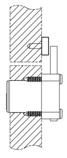
Lock is shown in locked position for standard drawer applications.
