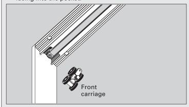
d) Secure the carriage to the cassette with the M5 pan head machine screw.
