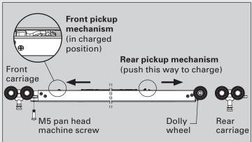
To load the SofStop mechanism into the track:
