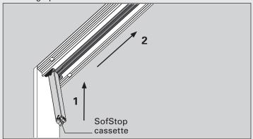
c) Slide the front carriage into the track with the tow bar facing into the pocket.
