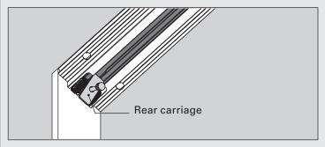
b) Insert the cassette into the notched end of the track, dolly wheel first, ensuring that the pickup mechanism is facing up.
