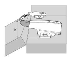
For all hinges with a straight hinge arm and a 3 mm spaced mounting plate. Including: Profile door hinges 95° and a 0 mm spaced mounting plate.
