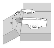
For all hinges with a straight hinge arm and a 0 mm spaced mounting plate. Exception: Profile door hinge 95°.
