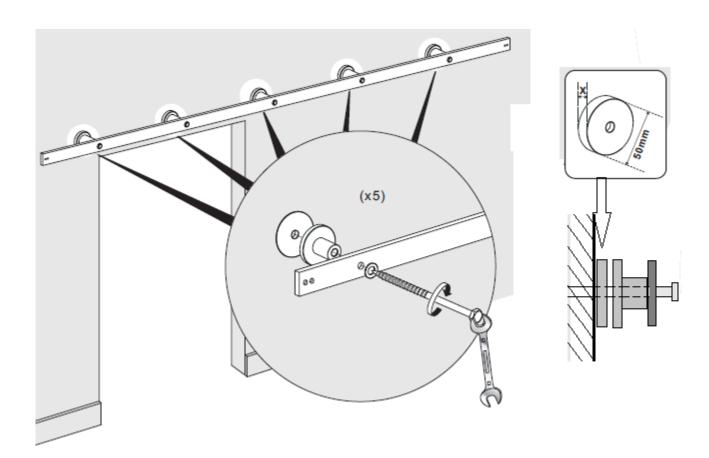
Insert Spacer Disc if necessary to shim track further from the wall. Select from 6mm and/or 12mm thick Spacers If a more pronounced spacing was necessary, are also available in suggested products:
