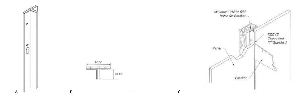
All recessed/ concealed « T » standards should be mounted right side up as shown by the "top" stamp (A). Before mounting, line up each standard using the bottom of each bottom slot as the guide. Once aligned, makes sure to fasten to a secure wall stud (or equivalent blocking) using appropriate screws (C). Make sure to utilize each screw hole. Please note that a minimum 3/16" by 5/8" notch is required in the stud or blocking to allow installation of brackets.
