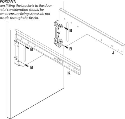
Fit door brackets to door using bracket screw positions.
