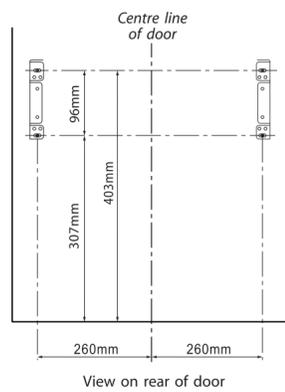
Calculate centre line of door and use above measurements to mark door bracket screw positions.
