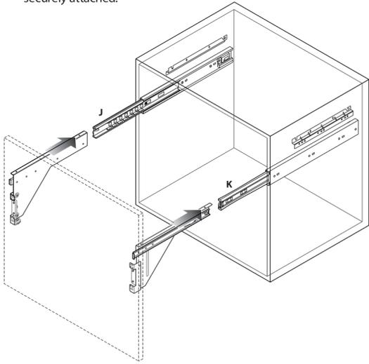
**6** Fit the frame to the runners using screws **c**
