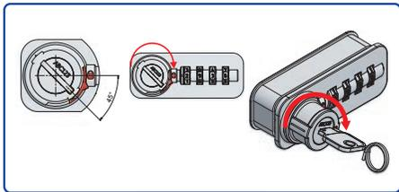
Press the programming pin into the knob (for example with the code tool or a ball-point pen) and, with the programming pin held down, rotate the knob by approx 45° until stop. The code tool is no longer required.
