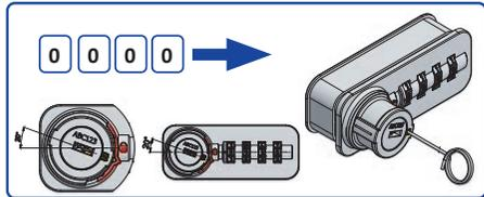
Press the programming pin into the knob (for example with the code tool or a ball-point pen) and, with the programming pin held down, rotate the knob by approx 20° until the arrow at the base of the knob is aligned with the red triangle on the lock case. A slight resistance can be felt. The code tool is no longer required.
