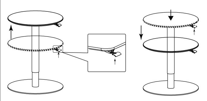
Lift the paddle for lifting the table top.
