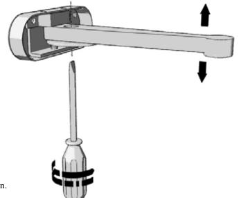
Insert the support and the disk. Next, attach and adjust the height with the pin.
