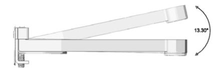
With the eccentric you can adjust the slope of the bracket upwards to a maximum of 13.30 degrees.
