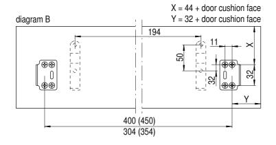
4 Assembling "frontis plate" Attach the "frontis plate" as indicated in diagram B. Fasteners: panhead screws 4.0 x 16
