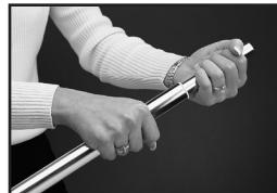
Loosen upper shaft by twisting counter clockwise just enough so that shaft will slide up and down (about 1/2 turn). Holding down on bottom shaft with one hand, extend upper shaft and engage over center pin in upper mounting plate, twist clockwise until tight.
