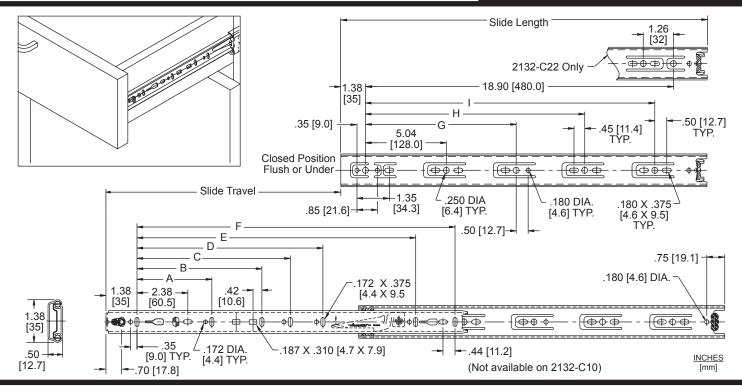
.50" +.062 / -.000 (1/2" +1/16" / -0) Available in clear electro-zinc (C), or black **Side Space Finish** [12.7 mm +1.6 / -0.0] zinc (CB) Even lengths 10"-28" [250 mm-700 mm] Mounting Side, optional face frame brackets Length Movement Steel ball bearings **Travel** 3/4 extension 75 lbs.\* [34 kg] per pair Also Drawer member cam action vertical Load adjustment, lever disconnect, positive stop, Height 1.38" [35.0 mm]
