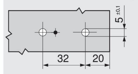
Fix with additional screw if used with wide angle hinges
