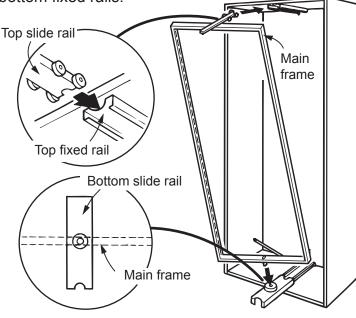
Align the main frame to the bottom slide rail groove in the right direction.
