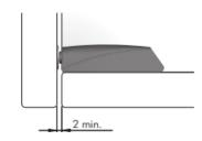
WITH BUFFER for cabinets using sprung hinges.
