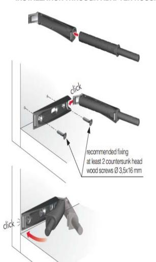
WITH MAGNET for cabinets using unsprung hinges or negative hinges.
