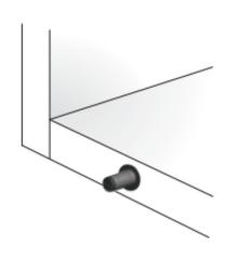
WITH MAGNET for cabinets using unsprung hinges or negative hinges.
