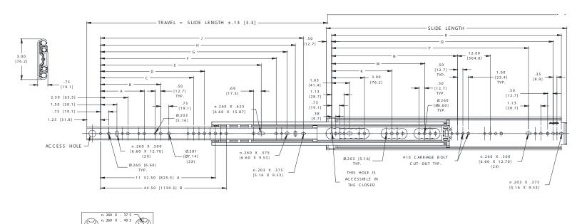
Note: Maximum screw head of .190" [4.8mm] high by .500" [12.7mm] diameter necessary to clear traversing members.
