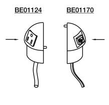
Snap the two halves together and drop into the 3" hole. Optional: For a tighter fit, apply doube-sided tape between the two sphere halves.
