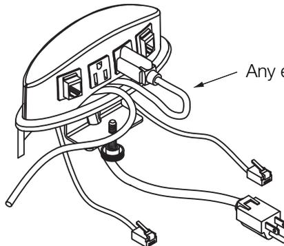
Snap the PDC housing into the base
