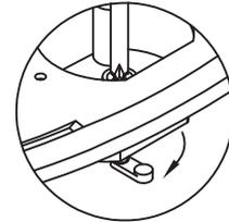
Use a phillips head screwdriver to tighten locking cams and secure PDC base into work surface.
