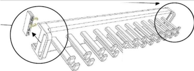
These pull-outs are easily reversible for right or left installation. To change mounting side, simply remove the end cap and insert it into the opposite side (see instructions for more details).
