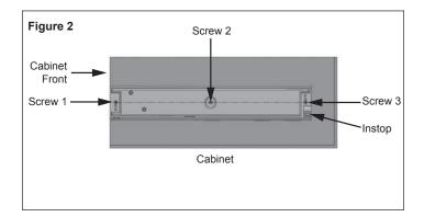
To modify angle, remove screws 1 and 3 and rotate around screw 2 to desired angle and reinstall, as shown in Figure 3.
