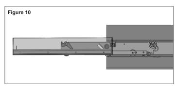
WARNING: Locking lever must be unlocked to remove drawer.
