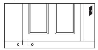
18. Roll door back far enough to mount T-Guide. If this means rolling off the end of the track, ensure door weight is supported using a block.
