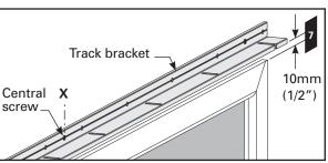
**Note:** There must be a 10mm (1/2") gap below the bottom of the mounting bracket. Cut architrave if
