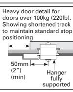
A heavy door may distort the hanger under load. If you are using a heavy door, preload/offset the hanger by applying firm pressure with the palm of your hand to the top of the hanger while it is fitted to the door.
