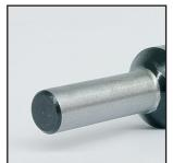
Shank design: Up to a diameter of 10 mm, cylindrical, like drill diameter; from a drill diameter of 11 mm - 20 mm, the shaft diameter is 10 mm; from a drill diameter of 22 mm - 32 mm, the shank diameter is 13 mm
