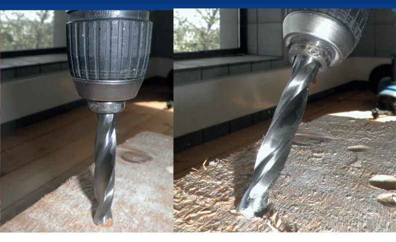
The HSS wood twist drill is made of high-quality chrome steel and, in addition to the centre point, it is equipped with 2 main cutters and 2 spurs as well as with a ground back guide.
