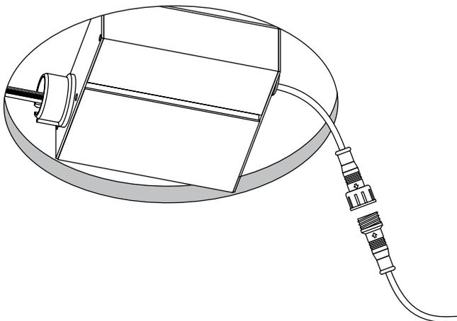
**4** Compress the springs and push the fixture in the opening. It is easier to do one spring at a time.
