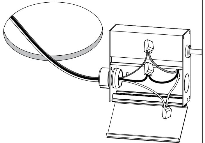
**3** Route junction box through cut-out and connect recessed LED panel to junction box with the quick connector.
