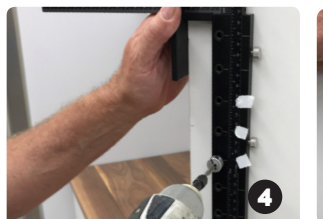
Mark your holes with tape for reference, drill first set of shelf pin holes
