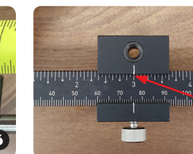
Transfer hardware measurement from step 6 to Sliding Drill Guide and tighten
