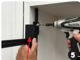
Set Large Stop to 37mm (industry standard). Drill top hinge plate holes
