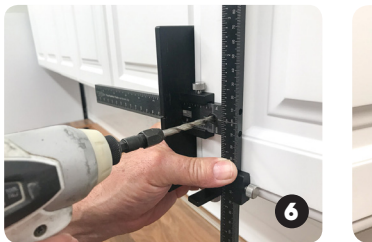
Position tool with stops as shown and drill hole through drill bushing
