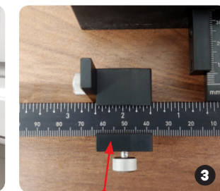
Set Sliding End Stop to measurement from step 2 and tighten
