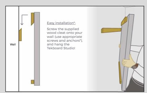
\*Wall cleat to be installed by customer; anchors, screws and holes are not included.
