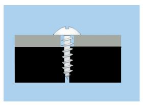
• Test applications for unforeseen complications, such as expansion/contraction issues (note: different colors react differently to heat). King StarBoard® ST contracts and expands at a rate of 6x10<sup>-5</sup> in./degree F, changing approximately 1/32 inch for every foot of length or width over a 40-degree temperature range.
