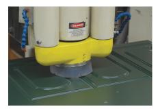
• With a 1/2" diameter router bit, feed rates of 12-16 feet per minute are normal. Rates must be slower for material that is 1/2" thick or thicker. Larger bits have higher tip speeds and RPM adjustments may be necessary.
