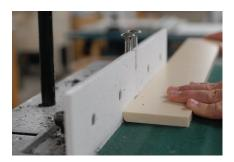
Edges may be finished with a router. Sanding may be used, but a very find sandpaper is required to avoid creating small, hard-to-clean scratches.
