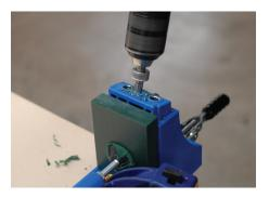
Use standard fasteners with oversized holes. Drill pilot holes first, followed by an oversized hole to allow for expansion and contraction. Use press-in threaded inserts for applications where repetitive motion is expected, such as a door hinge.
