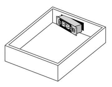
**Step 6 -** Align arms. With the drawer mostly closed, mark the position of the rear mounting bracket. It is important to make sure the drawer moves freely in and out and that the arms are square and even. Spend sufficient time at this step before fastening the bracket to the rear wall to make sure everything is square and the arms are in the correct position. Once that is done, secure with the 3 rear mounting bracket screws provided.
