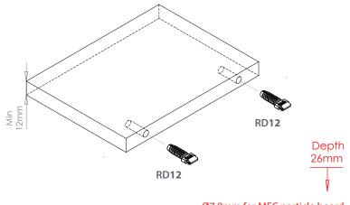
Ø7.8mm for MFC particle board Ø 8mm for other board types
