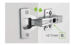
Independent side adjustment Acting on the "B" screw it is possible to change the amount of the door covering on the side of the cabinet.
