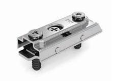
Metal linear mounting plate. Fixing by Expanding dowels Ø5mm. Independent vertical adjustment with CAM.
