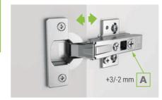
Depth adjustment Acting on the "A" screw it is possible to adjust the distance between the side of the cabinet and the door.
