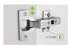
**Vertical adjustment**Acting on the "C" screw of the mounting plate it is possible to adjust the door vertically.
