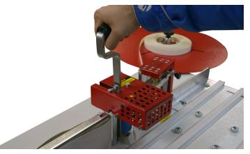
According to the first couple tests you will find an ideal amount of glue that must pass onto the panel. In case you notice that the tape is easily peeled off from the panel, try increasing the amount of glue or there may be an excess of glue, you'll notice an excess on the sides of the tape. To adjust the glue thickness, do the following:
