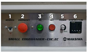
1. Main Power Switch (1): This Switch energizes the machine's control panel, without turning on the function.
