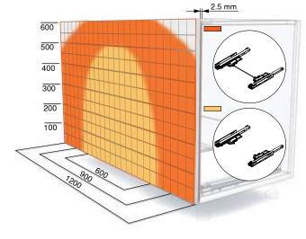
Shown in the diagram by way of example for height C, nominal length 500 mm with front stabilizer
