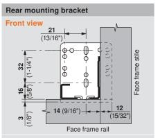
NOTE: For frame applications, use a minimum of three screws per bracket
