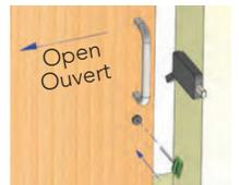
**Note:** Standard barn door to wall clearance is approximately 3/8" to 1/2". Install additional spacer as needed behind the strike faceplate if the door to wall clearance is over 1/2". Additional spacers can support maximum clearance of 3/4" between door and wall.
