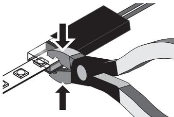
8. Push on the plastic cover to close it. Use pliers to clip the connector completely close until you hear a clicking sound indicating the connexion is good. Cover clips are on both sides of the KLIPR connector.
