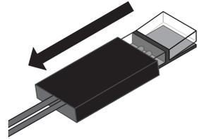
5. Gently slide the heat shrink tube over the connector until it is passed over the wires, be careful not to accidentally close any still open cover.
