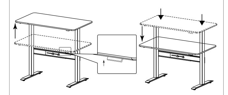
Lift the paddle for lifting the table top.
