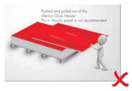
Stack the panels carefully, placing a protective laminate over the top and under the bottom panel. Usually Matt Meister panels are stacked in lots of upto fifteen, with one sheet of 2mm or thicker laminate each at the bottom and similar laminate on the top.
