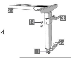
Depending on your installation, you can attach the Lower Brackets (part 2a) and the Center Brackets (part 2b) to the wall first - level and at the proper distance. Or, you may choose to attach the Lower Bracket (part 2a) to the Leg (part 1) with four (4) M6x14 Machine Screws (part 11). Attach the Center Bracket (part 2b) to the Leg (part 1) with four (4) M8x10 Machine Screws (part 14). Do the same for the other Leg.
