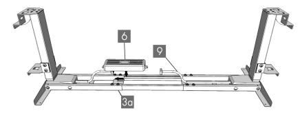
Slide the Control Box (part 6) onto the Frame End-CB (part 3a). Connect the cable exiting the Leg (part 1) that is attached to the Frame End-CB (part 3a) directly into the Control Box (part 6). Connect the Cable (part 9) to the other Leg (part 1) and to the Control Box (part 6).
