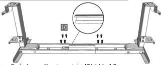
Set the base to the proper width and lock the position of the Center Rails (part 4) using eight (8) M6x10 Machine Screws (part 10).
