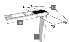
Place one of the Legs (part 1) into the Frame End-CB (part 3a) ensuring that the bar (arrow) is on "top" in relation to the Leg (part 1).
