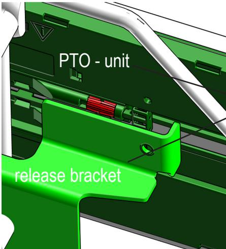
Ensure the release bracket hits the PTO counterpart without scratching any other parts. (If necessary bend the brackets to compensate)
