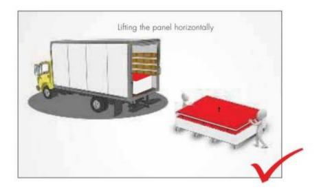
During material loading/unloading, ensure the panels are lifted cleanly and don't scrape or slide over each other.
