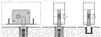
Locking with floor-mounted sleeve code 13787
