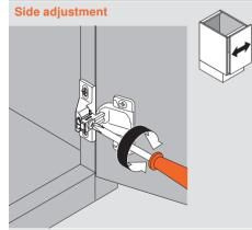
Side adjustment is possible on all COMPACT hinges. COMPACT 38N, 39C and 38C have cam side adjustment.
