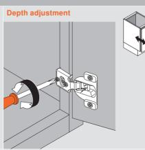
COMPACT 38N, 39C and 38C have cam depth adjustment
